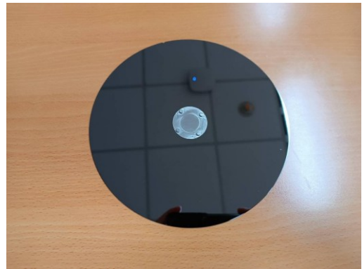
承載晶圓： 確認表面與晶背潔淨。 / Carrier wafer: confirm surface and backside cleanliness.
