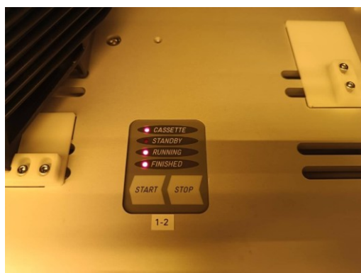
RUNNING 燈號 (閃爍)： Mapping 或處理中。 / RUNNING LED: mapping or processing is active.
