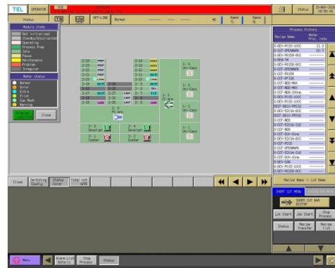
Status 畫面：監控設備配置與狀態。 / Status screen: monitor tool configuration and state.
