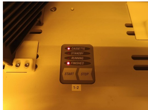
完成燈號：確認 FINISHED 後再取件。 / Completion LED: unload only after FINISHED is confirmed.
