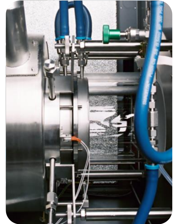
Water-cooled stainless steel flanges LPCVD前置水冷式法蘭
