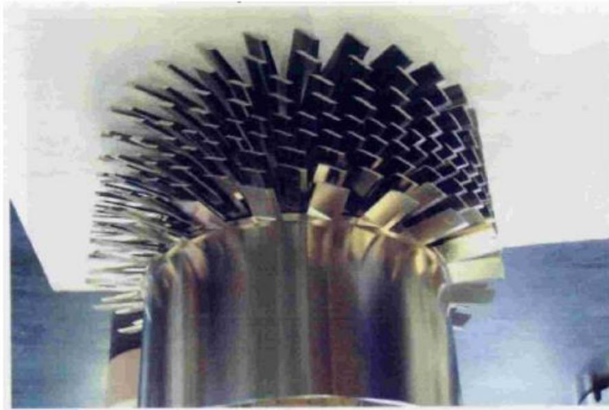
TMP rotor after using 18 months → Still working
